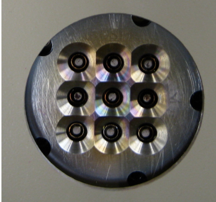
Figure 51. The thruster after operation. Note the discoloration on some of the emitter surfaces
