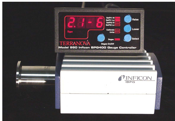
Figure 12. Pressure gage system for the vacuum chamber
