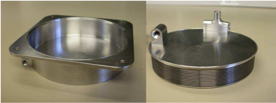
Figure 22. The propellant tank bellows before it was welded together, taken from Demmons [4]
