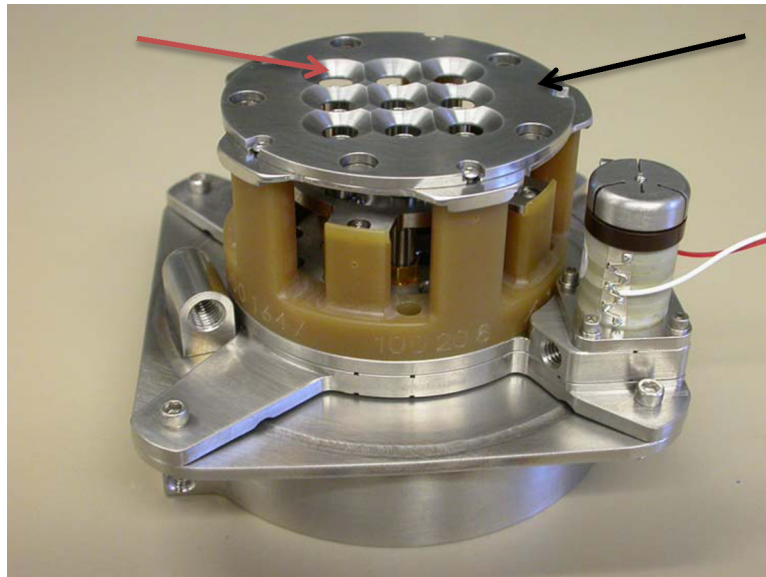
Figure 21. The round ring from the drilled holes is the acceleration grid, taken from Busek [1]
